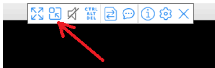
Fig. 3.83: Clicking on the Scale automatically icon
